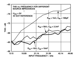
Figure 10. THD vs. Analog Input Frequency
