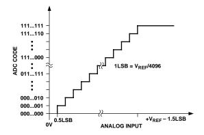
Figure 7. Transfer Characteristic
