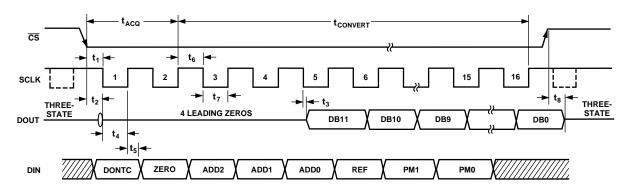
Figure 16. Serial Interface Timing Diagram
