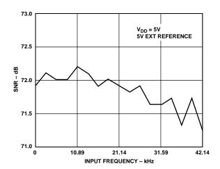
Figure 3. SNR vs. Input Frequency
