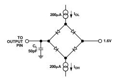
Figure 1. Load Circuit for Digital Output Timing Specifications
