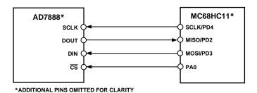
Figure 20. Interfacing to the MC68HC11
