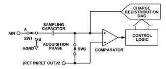
Figure 5. ADC Acquisition Phase
