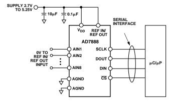
Figure 8. Typical Connection Diagram
