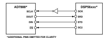
Figure 19. Interfacing to the DSP56xxx
