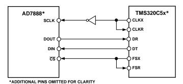
Figure 17. Interfacing to the TMS320C5x
