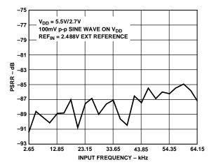
Figure 4. PSRR vs. Frequency
