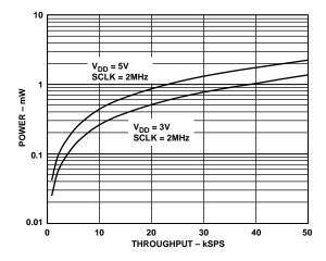
Figure 12. Power vs. Throughput
