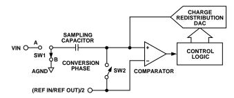
Figure 6. ADC Conversion Phase
