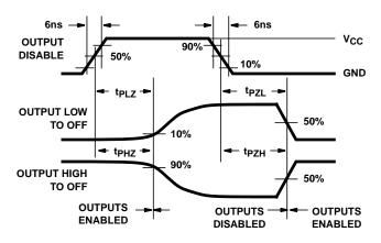
FIGURE 3. HC THREE-STATE PROPAGATION DELAY WAVEFORM
