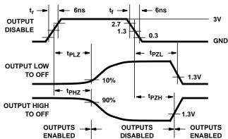
FIGURE 4. HCT THREE-STATE PROPAGATION DELAY WAVEFORM
