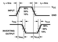
FIGURE 3. HC AND HCU TRANSITION TIMES AND PROPAGA-TION DELAY TIMES, COMBINATION LOGIC
