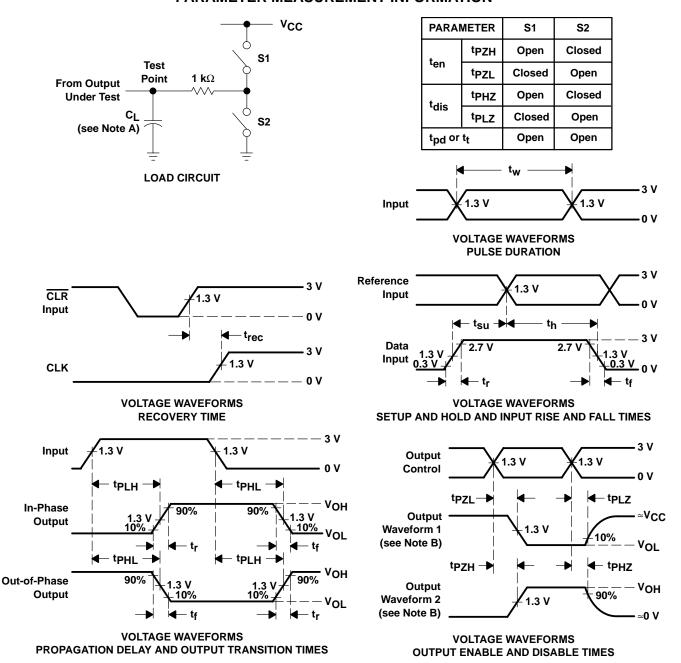
NOTES: A. C<sub>I</sub> includes probe and test-fixture capacitance.
