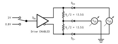
Figure 3. Differential Driver DC Test Circuit
