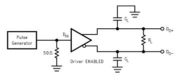
Figure 4. Differential Driver Propagation Delay and Transition Time Test Circuit
