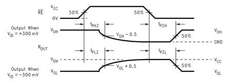
Figure 11. Receiver TRI-STATE Delay Waveforms
