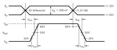
Figure 9. Receiver Propagation Delay and Transition Time Waveforms
