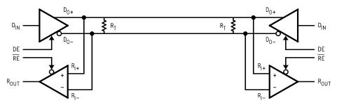
Figure 12. Bi-Directional Half-Duplex Point-to-Point Applications
